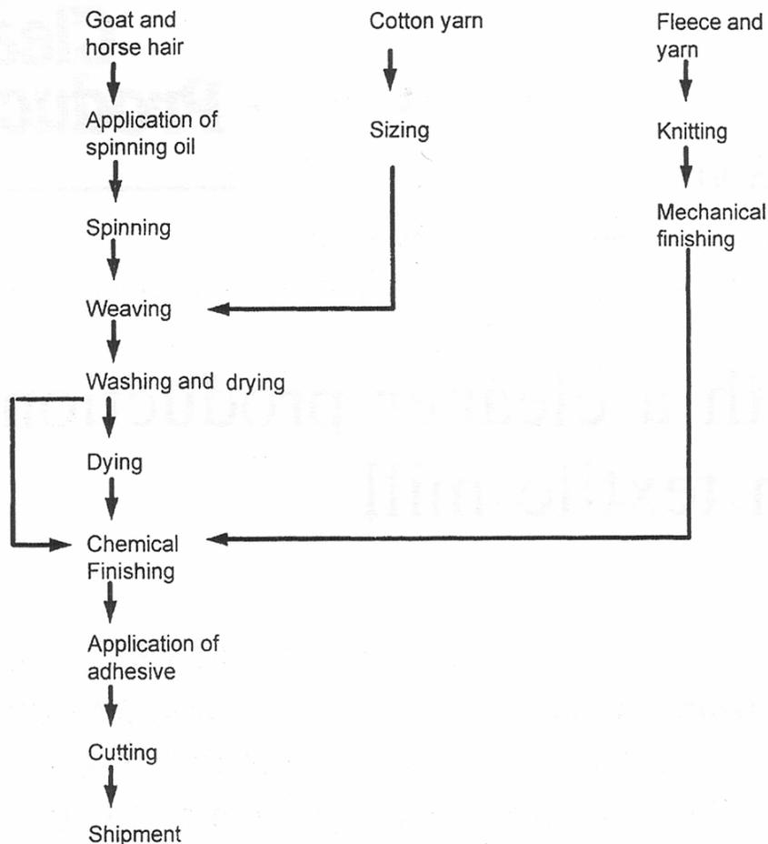
*Figure 9: flowsheet of the textile mill*
