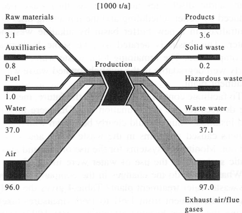
**Figure 10: Overview of the materials flows in the textile mill
