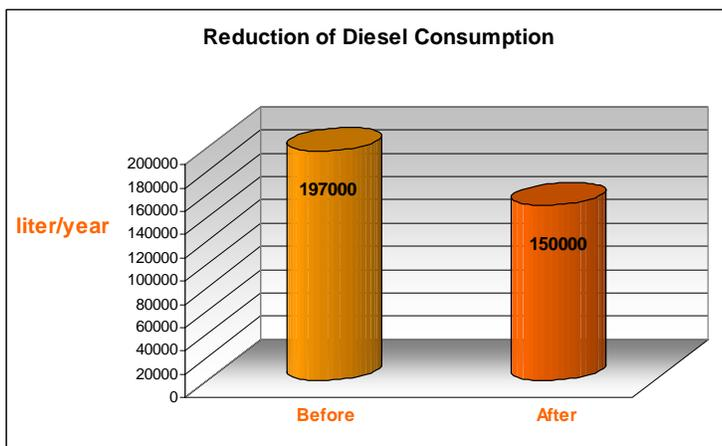
250 KVA, 8 years old generator were sold for 4000 USD and exchanged for a 500 KVA at 42000 USD new generator as a CP options at Sevenplast which is illustrated below:
